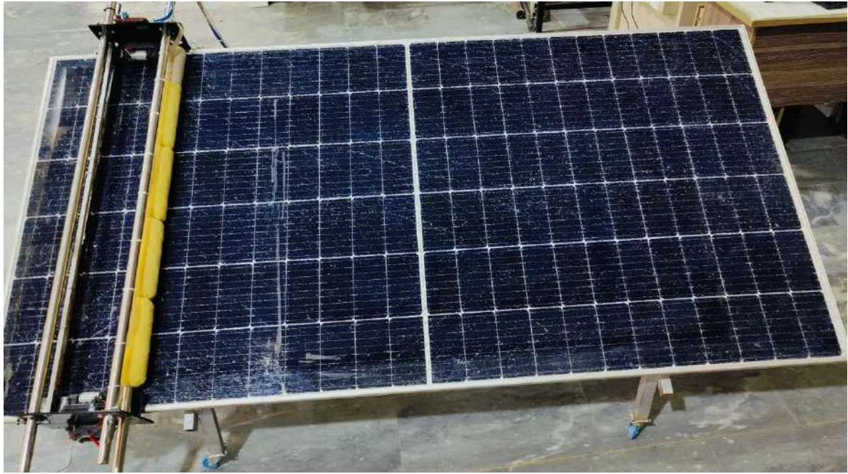
Figure 47 Solar panel after cleaning with Mechanism
