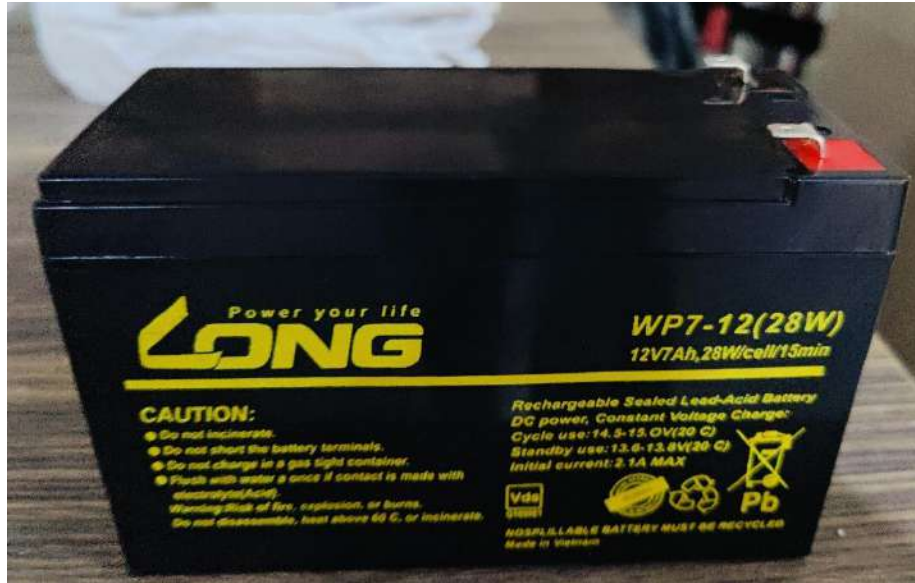
Figure 36 12V 7Ah Battery
