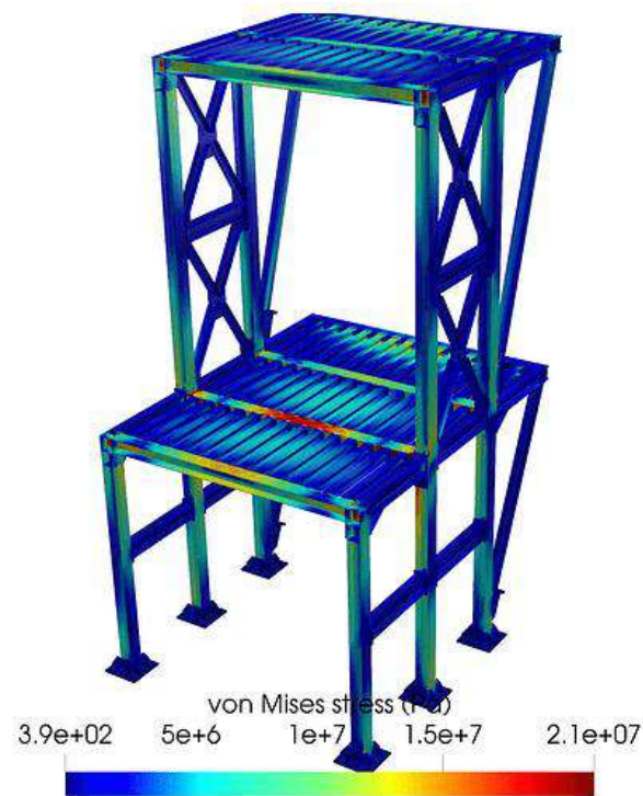
Figure 6-3: Von-Mises stresses of a Structure
