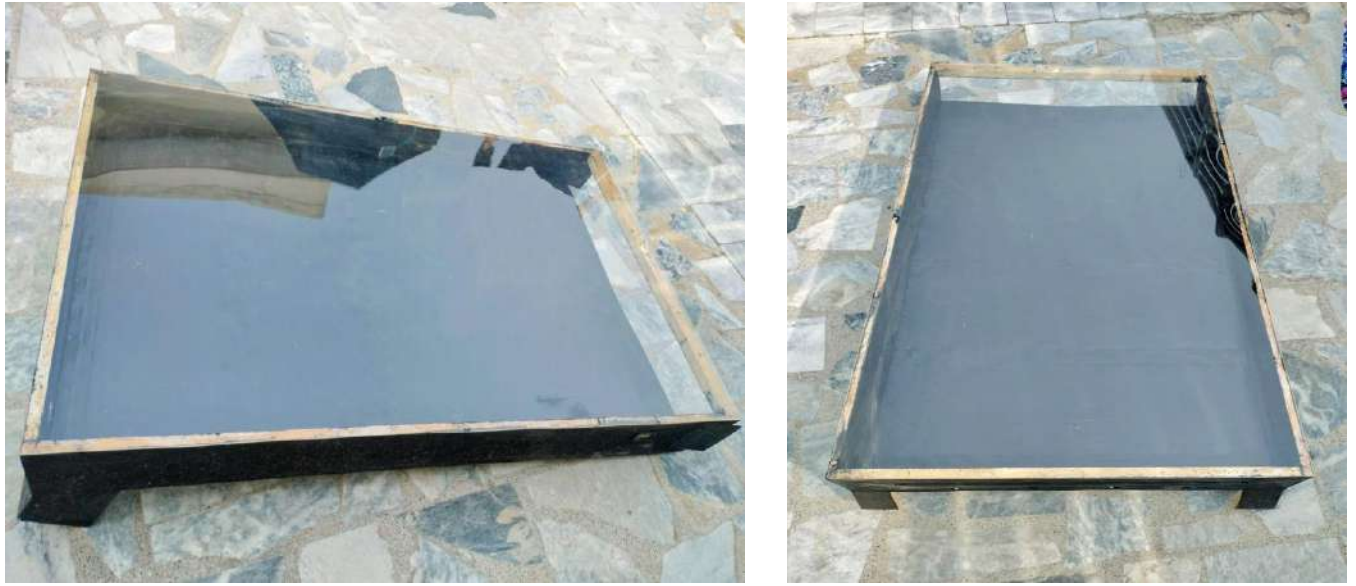
Figure 7-2: Fabrication of Inlet Chamber
