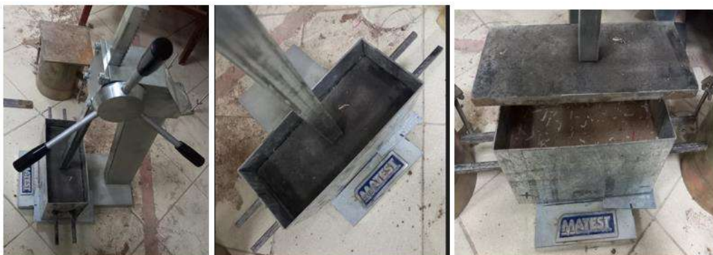
Figure 4.17 Compressing the sample batch to get compressed adobe
