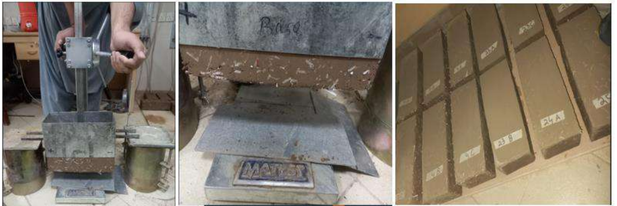
Figure 4.18 Demolding process of adobe from compression machine
