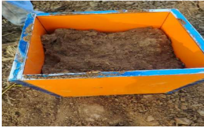
Figure 3.1 Undisturbed sample collection (UET NWL)
