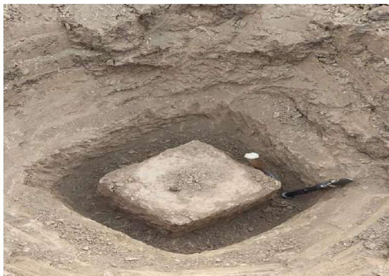
Figure 3.3 Preparing Undisturbed Sample (UET NWL)
