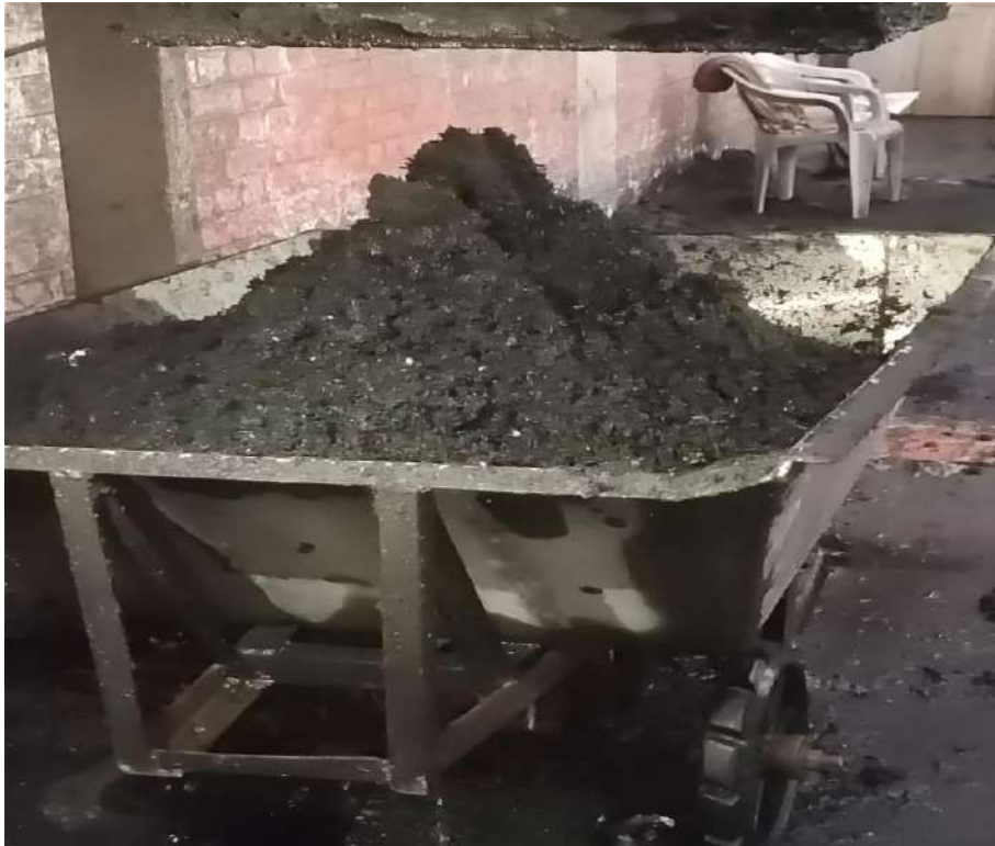
Figure 2.3 Rice Husk Ash after milling process (Source: Sapphire fabrics)
