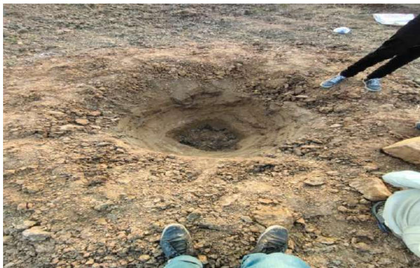
Figure 3.2 Sampling from 3 feet depth (UET NWL)
