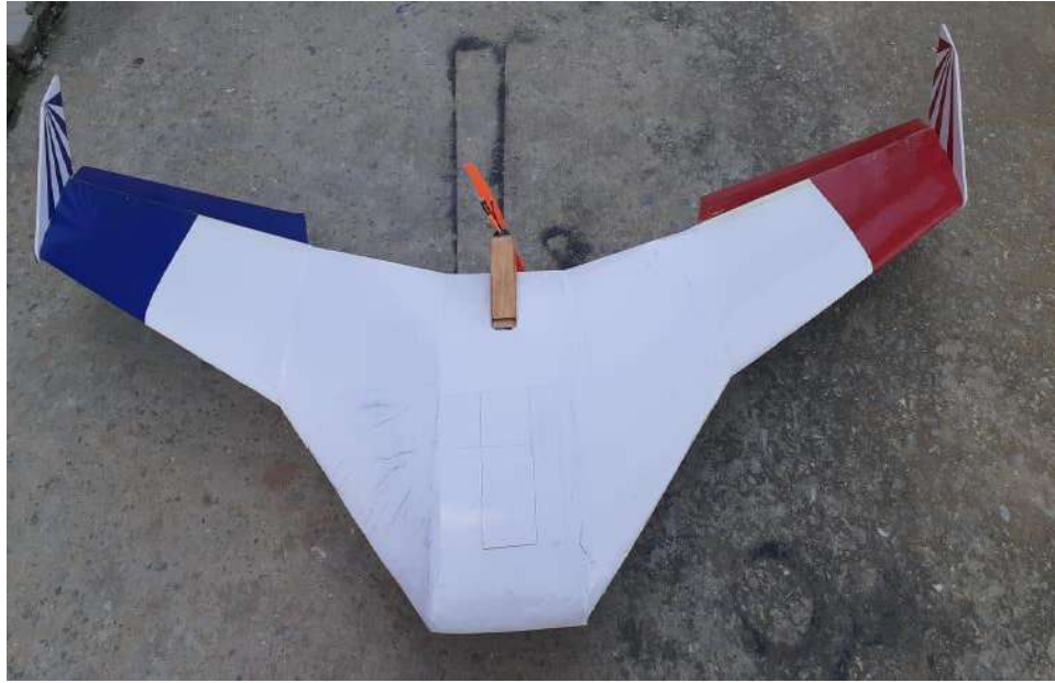
Figure 2: Blended wing body prototype
