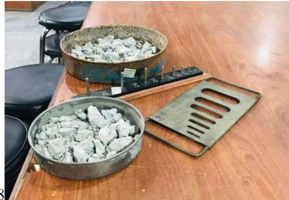
Figure 3.1 Sample of Demolished Concrete
