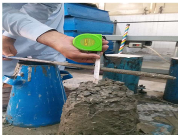
Figure 3.13 Slump Test for Concrete
