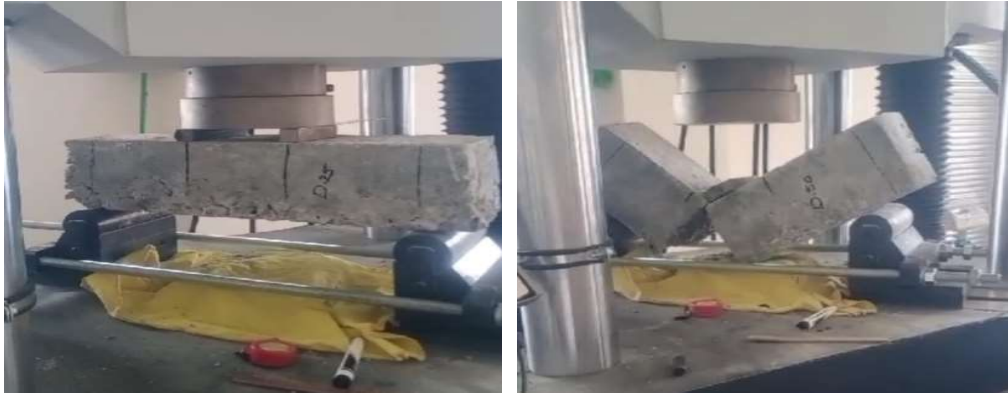
Figure 3.16 Concrete Sample Before and After Flexural Test
