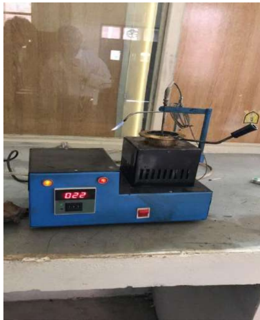
Fig 3.6.4:performing the flash and fire test
