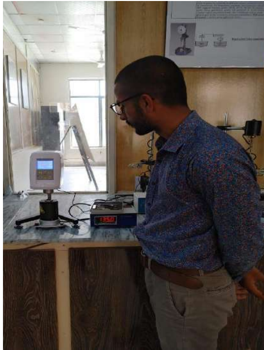
Fig 3.6.6:checking the viscosity of bitumen
