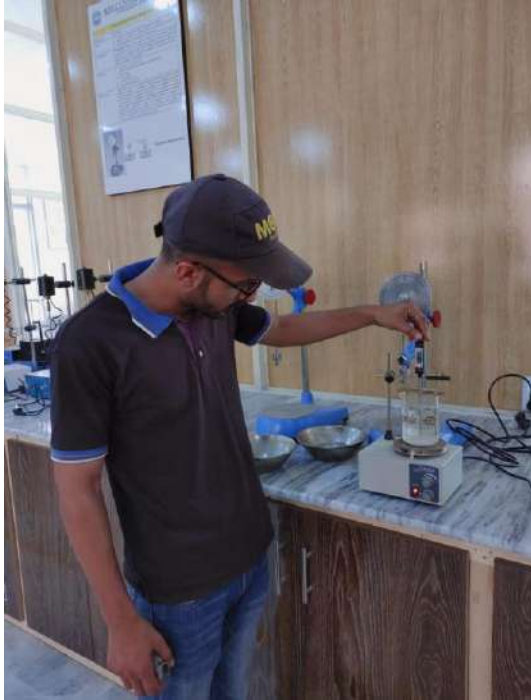
FIG 3.6.2:checking the temperature of water during softening point test
