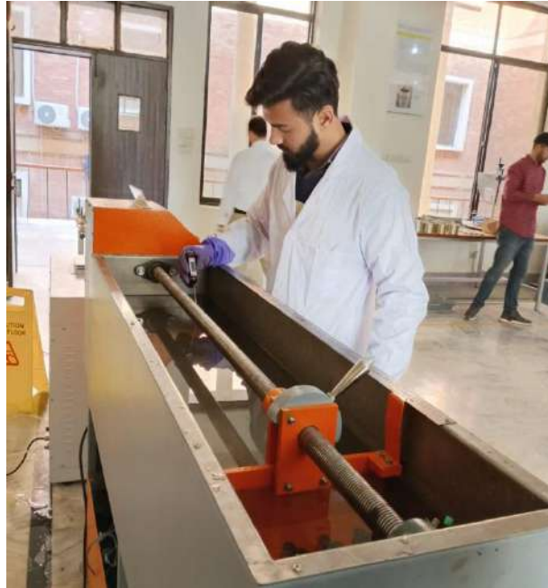
Fig 3.6.3: monitoring the temperature during ductility test
