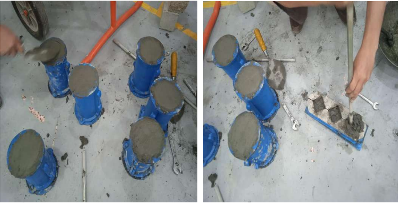
fig.3.1. (a) Casting of cylindrical and cubic mods
