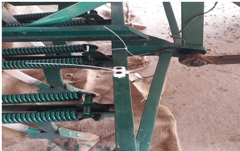
Figure 3.4: Position of the sensor on a conventional drill
