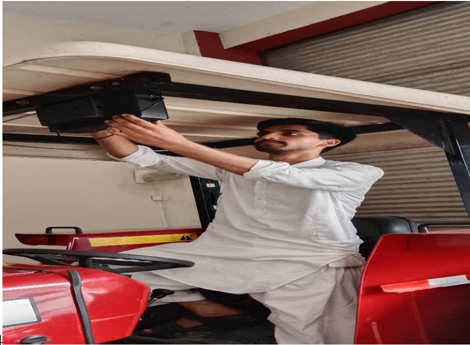
Figure 3.5: Installing Seed Depth Monitoring System
