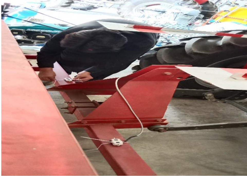
Figure 3.7: Manually measuring distance b/w sensor and plate for comparison with sensor reading
