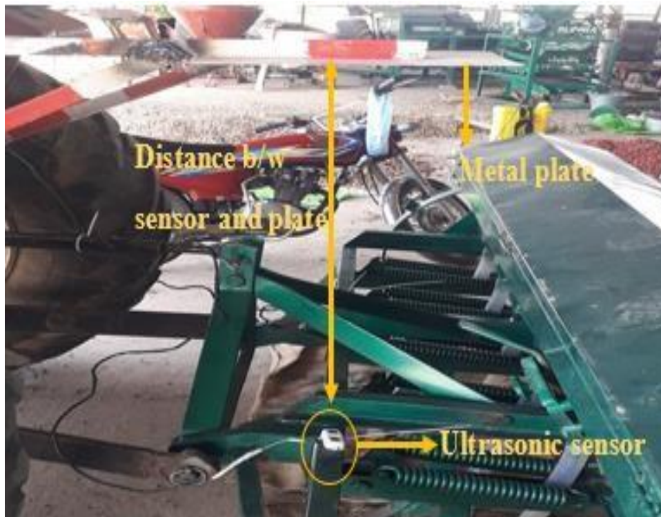
Figure 3.6: Positions and distance b/w sensor and metal plate
