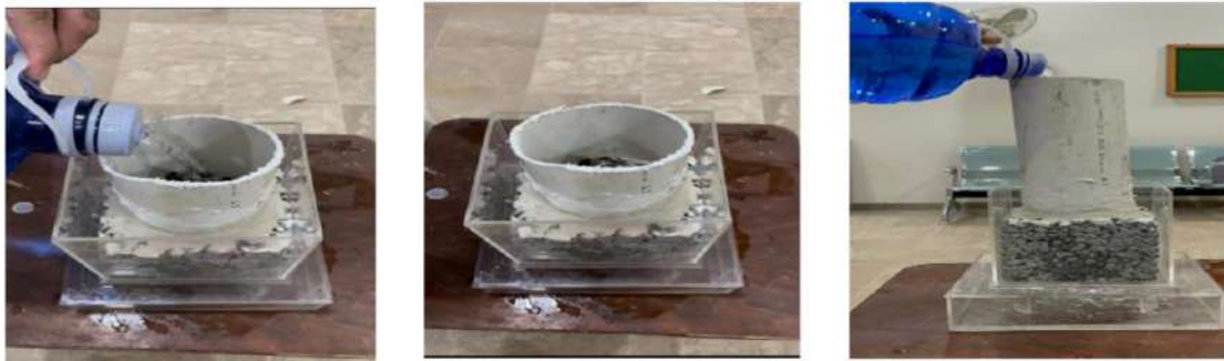
Figure 6: Operating water head test on pervious concrete
