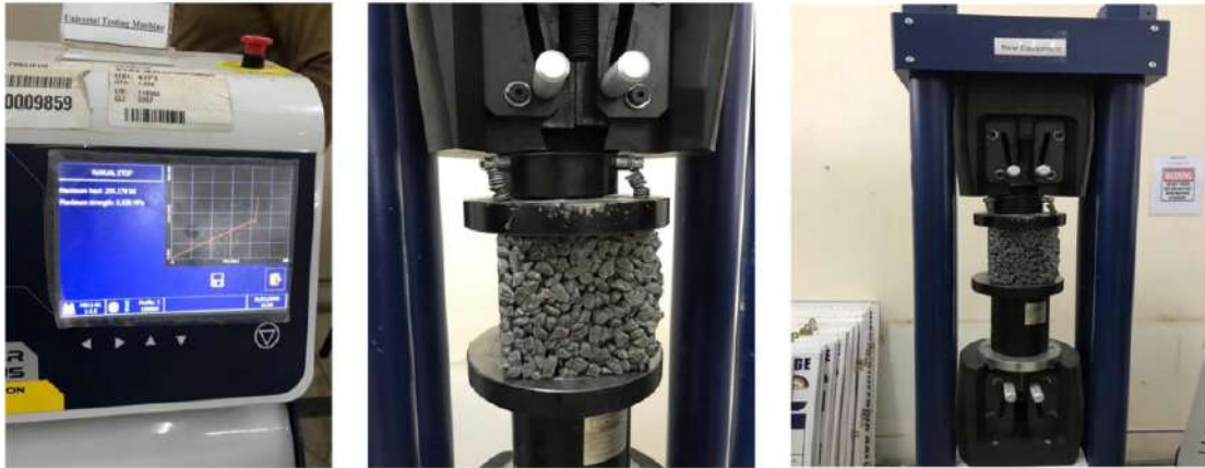
Figure 4: Compressive strength on pervious concrete using UTM (universal testing machine)
