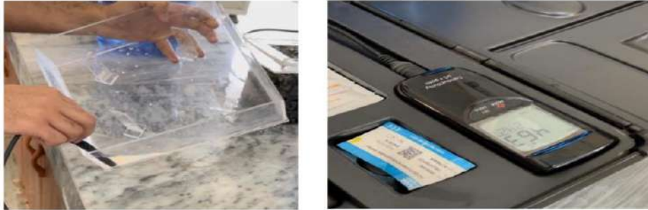
Figure 5: Electricity conductivity test on pervious concrete
