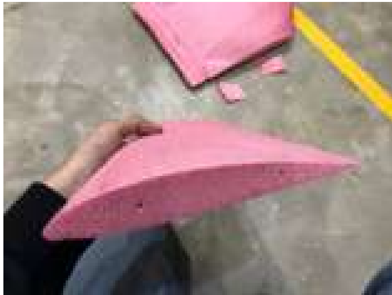
FIGURE 5.7: Wings cross section showing Airfoil
