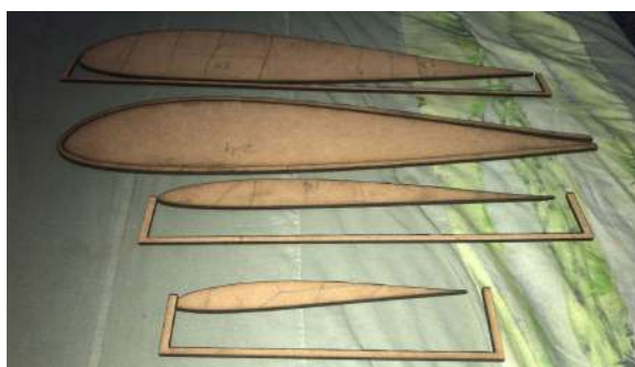
FIGURE 3.9: laser-cut templates for Airfoil
