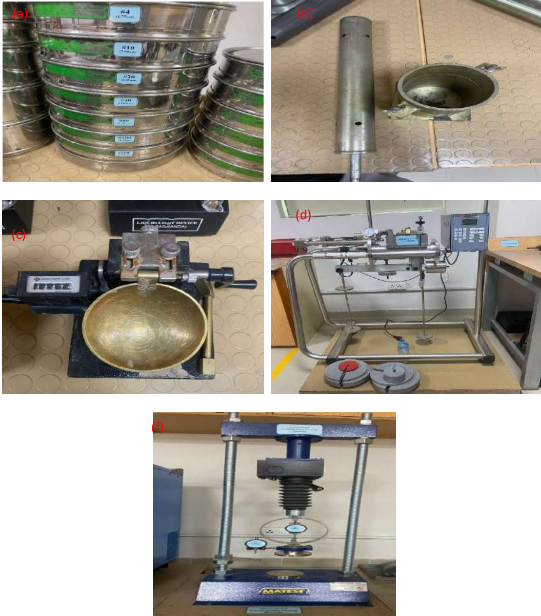
Figure 3.3 Tests to be performed: (a) Particle size distribution test, (b) Compaction test, (c) Atterberg limits test, (d) Direct shear test and (f) unconfined compressive test
