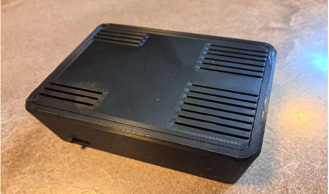
Figure 11: 3-D printed housing for climate monitoring node
