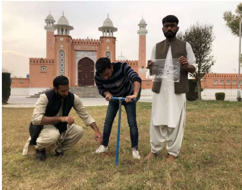
Figure 3.4: Soil Sample Collection
