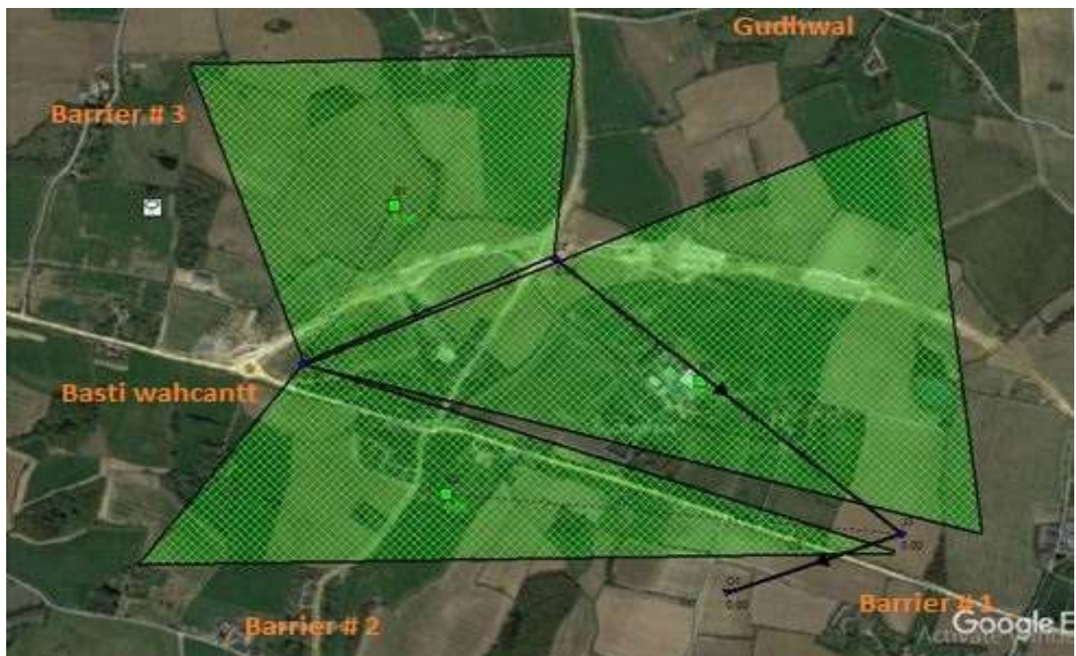
Figure 4.2: Drainage Area in SWMM
