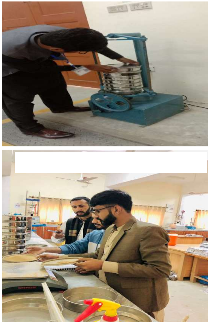
Figure 3.5: Taken during Sieve Analysis of soil sample
