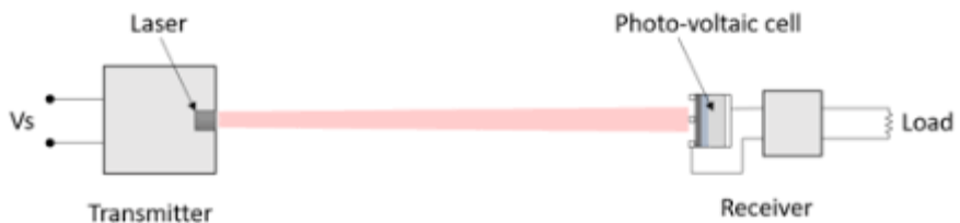
Figure 5 infra-red power transmission.
