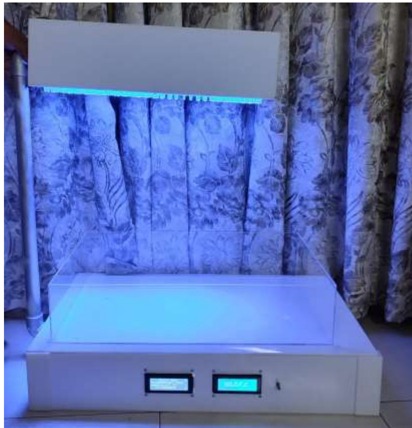
Figure 2.1: portable phototherapy device for neonatal care
